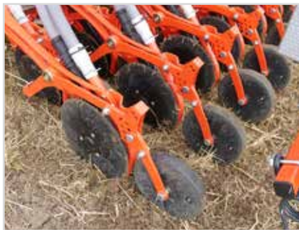
CX-II coulters with double entry for two sorts of application and seeding in one pass.
