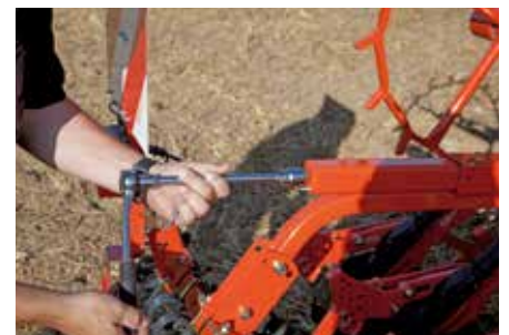
Depending on the soil conditions the pressure and angle of the following harrows can be adjusted manually.
