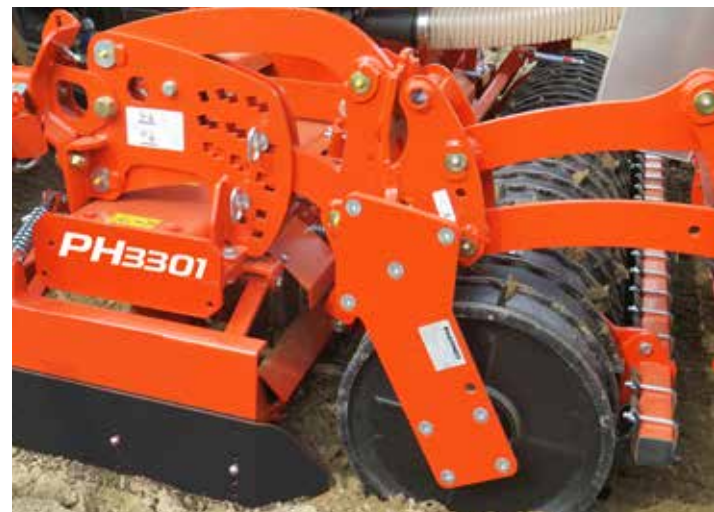
The coulters bar can easily disconnect to use the power harrow in solo operation e.g. on the headland.
