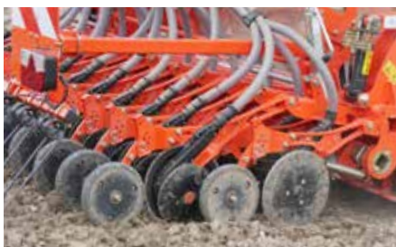
The Kubota CX-II coulters consist of two steel discs (Ø325mm) with 12.5cm or 15cm row spacing. Perfect depth control is ensured by the press wheels (Ø 250mm).
