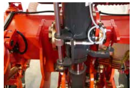
An intelligent two piece hydr. cylinder for best ground following.
