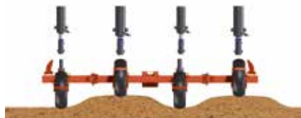
Intelligente and individual adaptation of the wheels due to the two-piece hydraulic cylinder.
