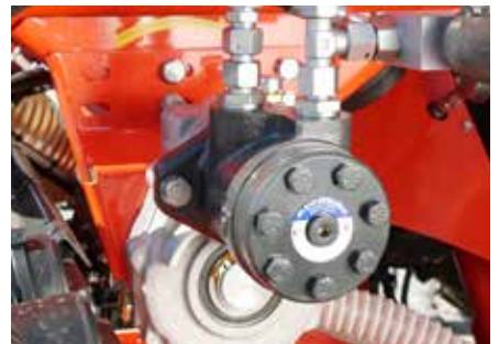
Optional electro-hydraulic drive for the fertiliser application. Fertiliser rate can be adapted even during work.
