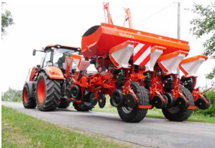
PP1601TF - Very compact in transport position. Designed for a transport speed of up to 40km/h with EU Type approval.
