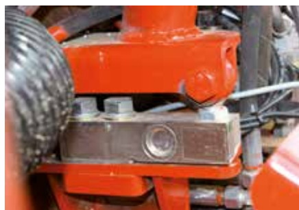
Weigh cells for the precise and controlled fertiliser application
