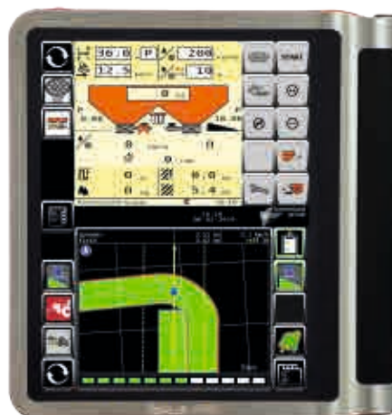
Automatic RPM warning on the terminal
