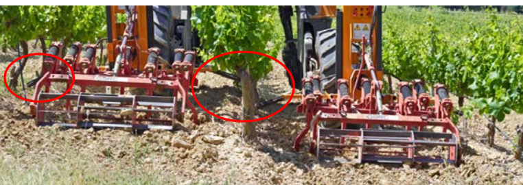
Centring probes on the tool holder arms
