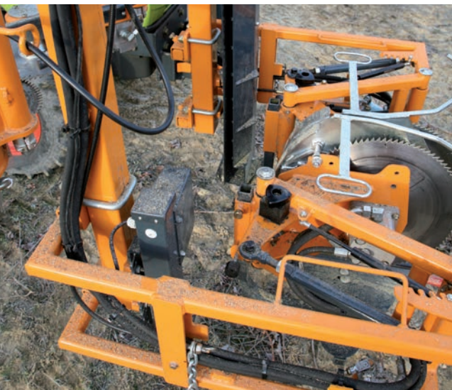
Automatic cordon tracking by vision system.
