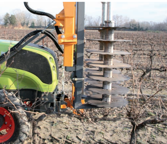
Precise adjustment of the discs for a clean cut
