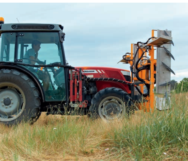
Reduced overhang, ideal for transport and at headlands
