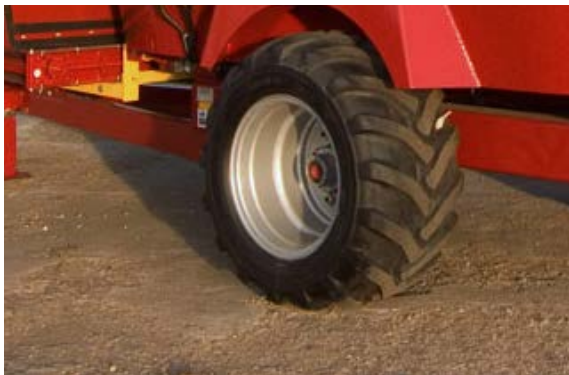
Flotation Tire Upgrade Upgrade to one of Supreme's flotation tire and wheel packages and you will be ready for varying types of terrain conditions from rough to soft and muddy.
