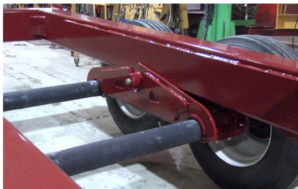
Tandem Axle Walking Beam Supreme's walking beam is designed to distribute and carry the weight of the processor through the tandem axle easily and effectively. Only available on 900T-1700TR.
